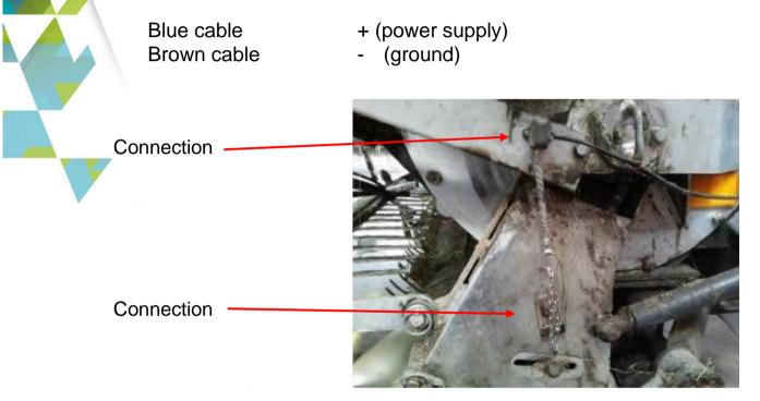
Connect the cord switch supplied to the cable provided (3 m long). Attach the cord switch to the pick-up of the harvester. If a pick-up signal is present this is connected to the blue cable (in this case the brown cable remains free).
